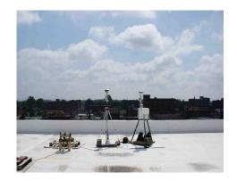
Site description: This is a center city population oriented FRM PM<sub>2.5</sub> and Carbon Monoxide site located in downtown Canton. This site has FRM PM<sub>2.5</sub> and continuous PM<sub>2.5</sub> monitors located on the roof of the Canton Health Dept. There is also a street canyon CO monitor situated on the second floor of the building. The land use is considered both commercial and mobile.
